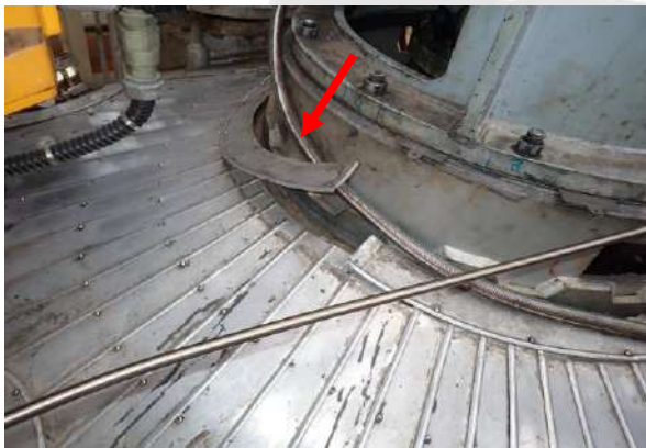
Found damage on insulation cover.
