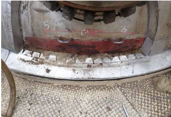
Found moderate corrosion on top head.(Depth= 1mm.)
