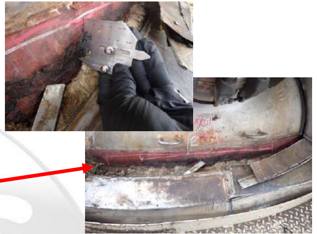
Found severe corrosion on top head.(Depth=3-7mm.)
