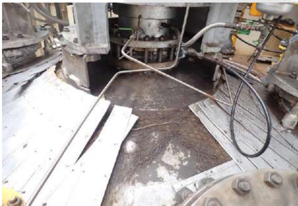
Found damage on insulation.
