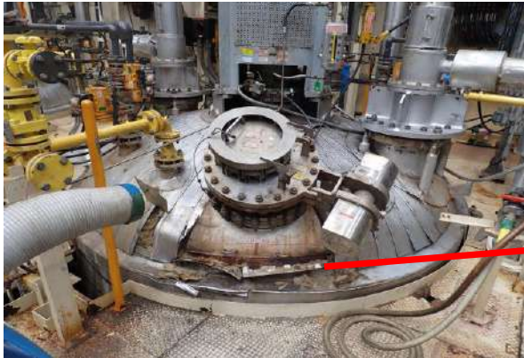
Found severe corrosion on top head.
