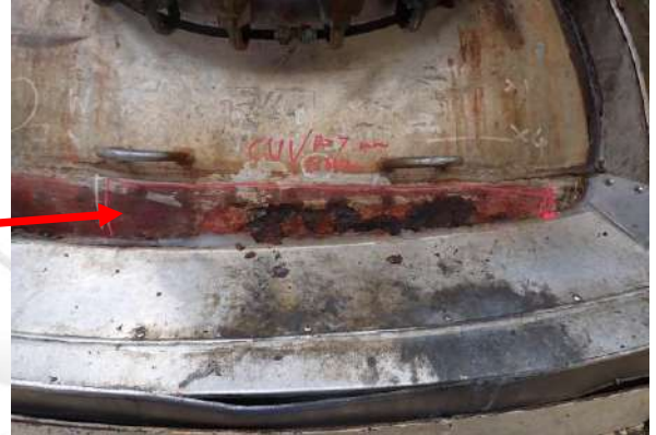
Found severe corrosion on top head.(Depth= 7mm.)
