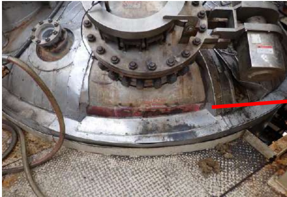
Found severe corrosion on top head.
