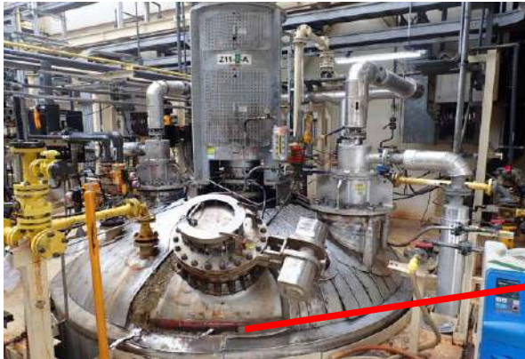
Found severe corrosion on top head.
