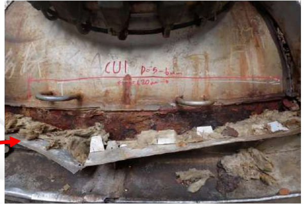
Found severe corrosion on top head.(Depth= 5-6mm.)
