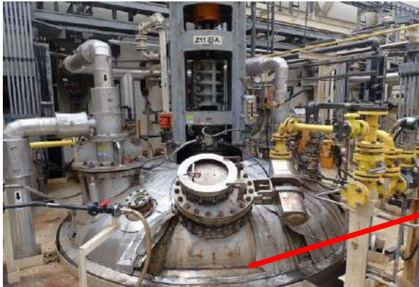
Found severe corrosion on top head.
