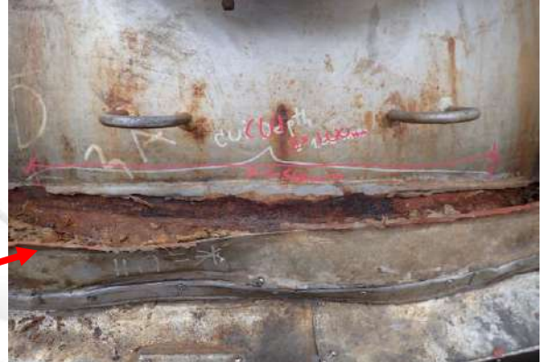
Found severe corrosion on top head.(Depth=1mm.)
